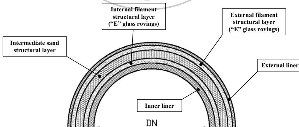
*Figure 1:* FWC pipes wall section.
